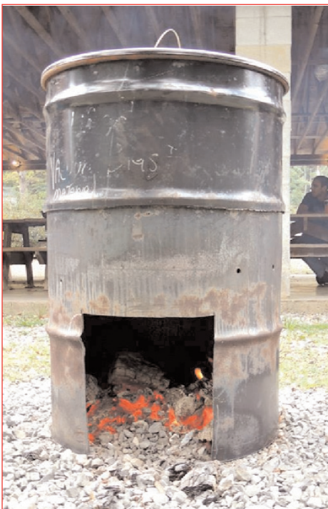
An oven constructed from a steel drum used to make "drum" bread.
